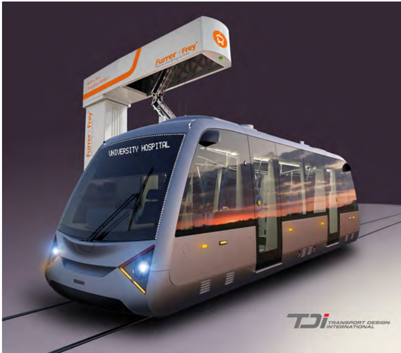
Figure 3: VLR Vehicle with Furrer+Frey All-in-One (AIO) opportunity charging station (Graphic: TDI).
